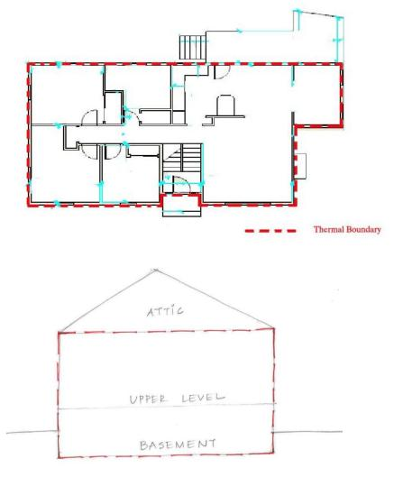
2. Hand draw the wall, roof and foundation assembly layers, from outside air layer to inside air layer. Show your calculated R-value for each.
